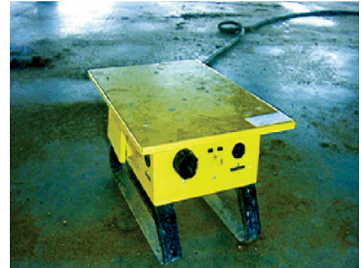
Typical “Spider box” supplies GFCI-protected receptacle for use on construction sites.
