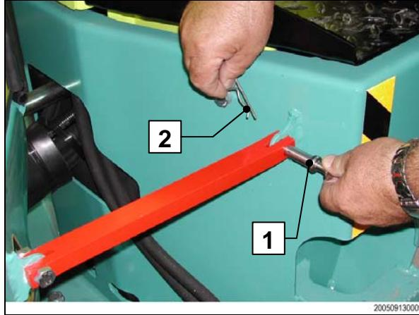
Now snap in the joint protection and secure it with the lock bolt (1).
