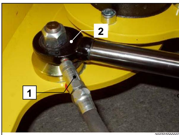
Clean the grease nipple before greasing.
