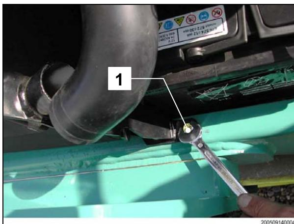
Unscrew the hood holder screws (1) on both sides of the roller.
