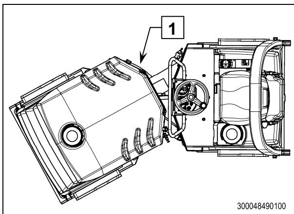
Turn the steering wheel all the way to the left so that you can easily access the engine oil drain (1).
