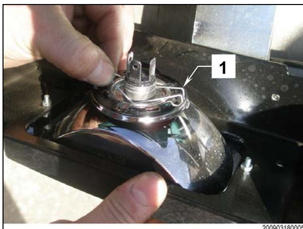
Press on the end of the securing clip (1) to remove it.
