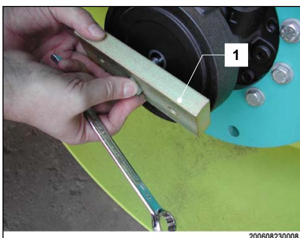
Screw the brake release chock (1) onto the drive motor.
