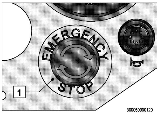
Now turn the emergency stop button (1) slightly in the direction of the arrow until it disengages.
