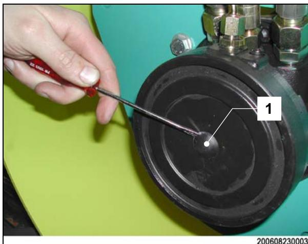
Remove the protective cap (1) on the front and rear drive motor.
