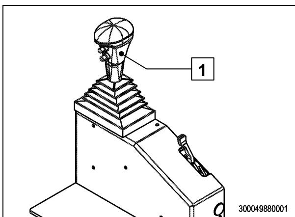
Move the drive lever (1) to zero position.
