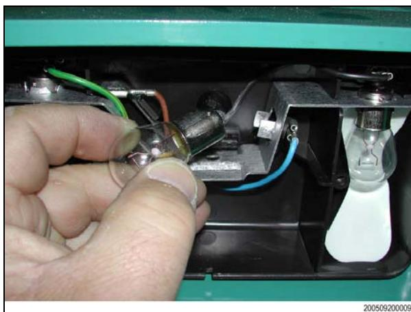
Replace the defective bulb with a new one of the same type and power.
