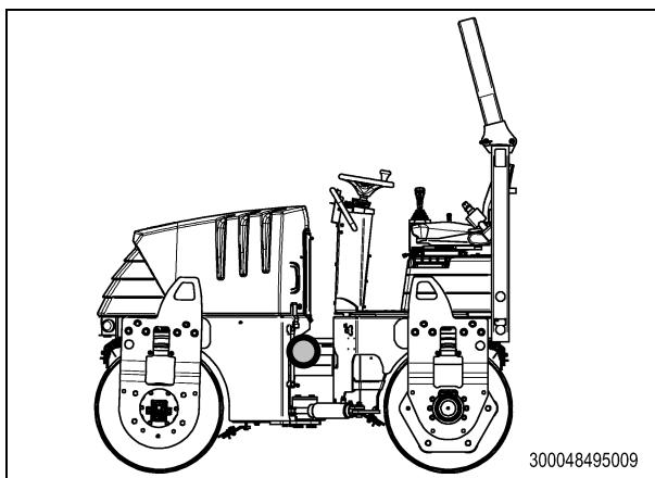
The center of gravity relevant to transport is located 710 mm from the floor and approx. in the center of the machine, depending on the fill level of the diesel or water tanks.
