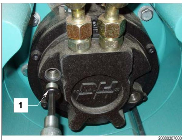
Remove the two cover screws (1) on the drive motor with an Allen key (SW8).
