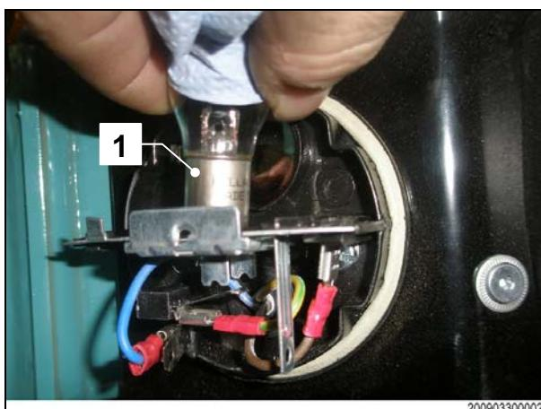
Replace the defective bulb (1) with a new one of the same type and power.
