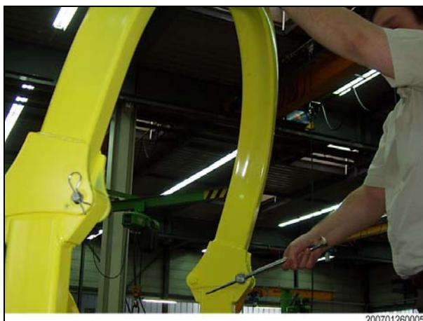
Both sides must be secured with bolts
