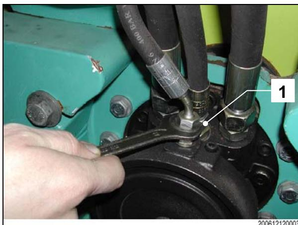
Remove the brake hose (1) from the front roller drum front drive motor.
