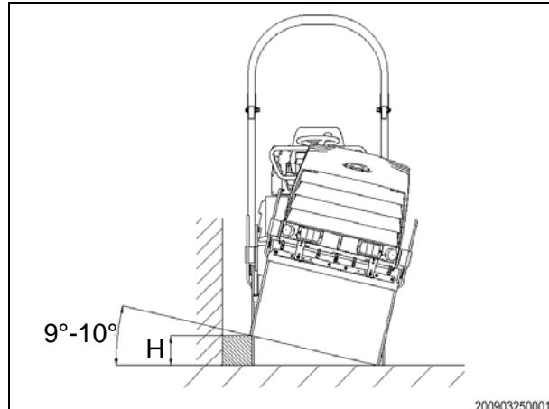
5. With the front wheel of the roller only, drive the side edge of the roller drum onto a solid, secure object with the following height H:
