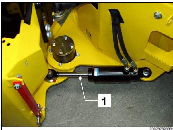
Rotate the steering to the stop to grease the cylinder.
