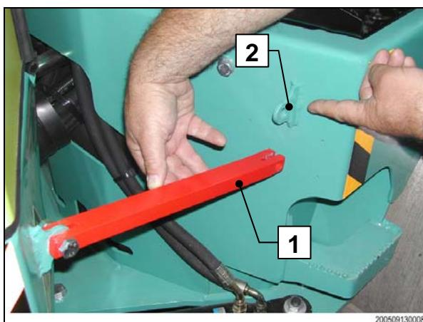
Carefully turn the roller steering wheel until the joint protection (1) comes in line with the opposite loop (2).
