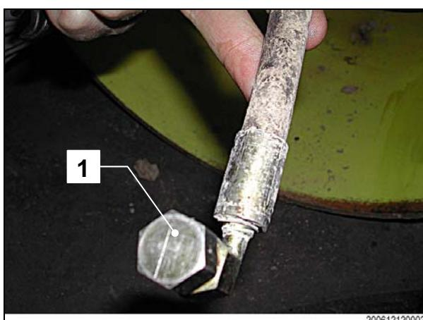
Seal the open hose end so that it can be pressurized.
